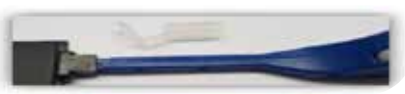
Cleaning tool with adaptor removed and the tip in a through adaptor for cleaning internal connector or a fiber port requiring cleaning
