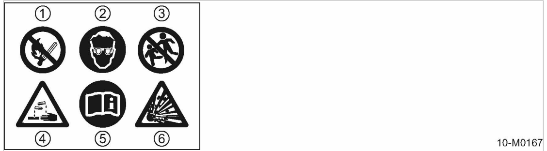
Fig. 43 Safety signs - warning stickers on the battery
