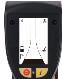
Active modes such as Metal mode, Bluetooth, GPS, and Points of Interest are shown on the LCD.
