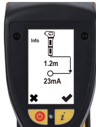
Press the i button for a depth reading with current measurement and logging options.
